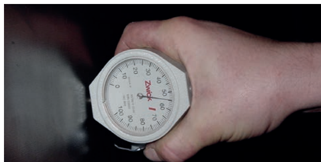
Measurement of Shore A hardness
