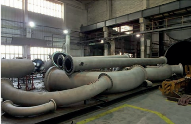
Rubber lined pipe parts after vulcanization in the autoclave
