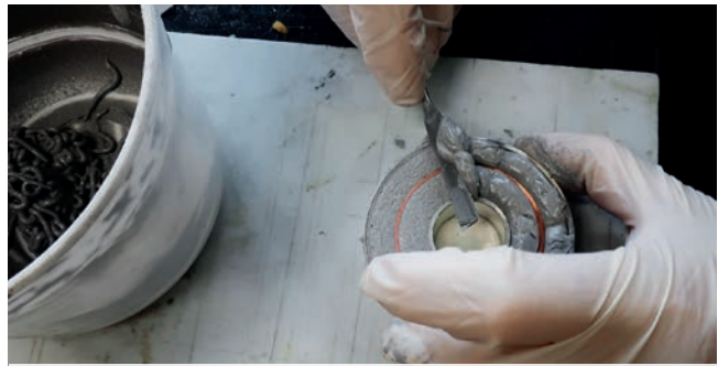
Molding and bonding a bearing seat
