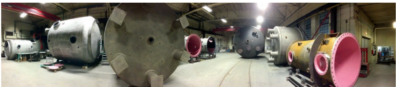
Workshop rubber lining in Warstein
