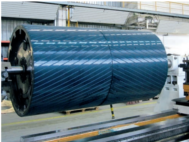
Drums coating with polyurethane
