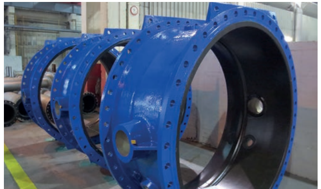
Rubber-lined flow-meter pipe
