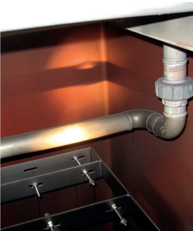
COROFLAKE coating in a wet ESP
