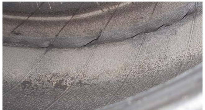
2.3.2 – Cracks in reinforced sidewall
